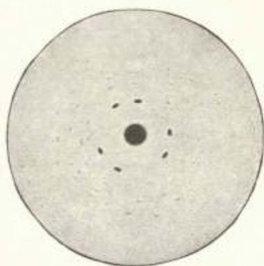
FIG. 16.—Laue effect for a zinc-blende plate parallel to a tetrahedral surface
